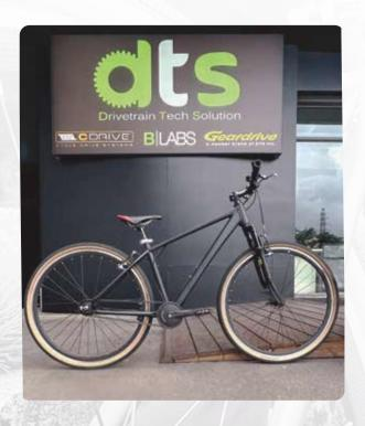
Cycle Drive Systems is a division of Delta Cycle Corporation, operating successfully in the U.S.A. since 1990 with a reputation for innovative design of useful bicycle accessories. In recognizing that the traditional roller chain with cog has changed little in 100 years, Cycle Drive developed it's unique matching toothed belt and precision sprocket system specifically for use on bicycles. This has been made available as Original Equipment for Manufacturers since 2008.
